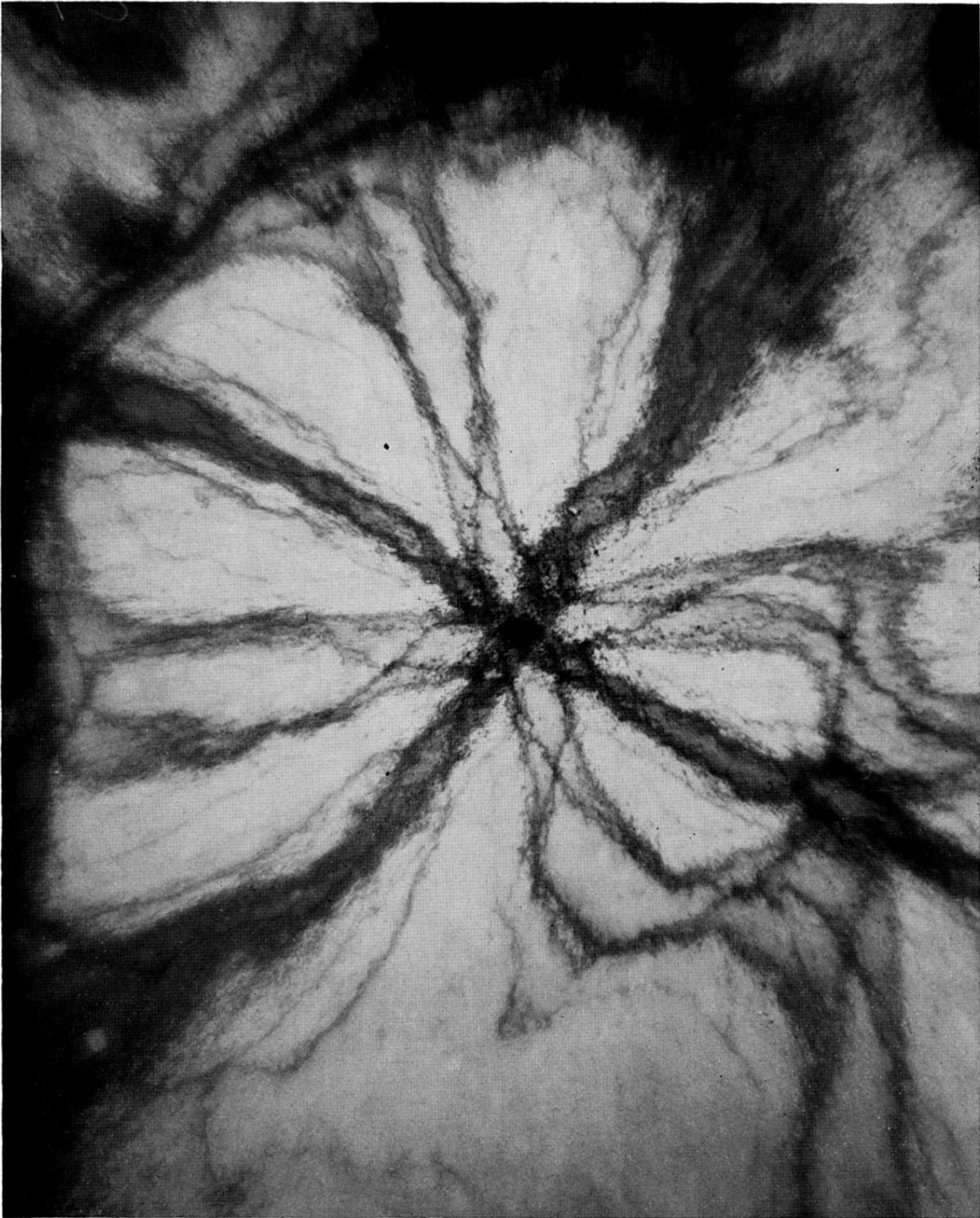
FIG. 2. Transmission electron micrograph of single-crystal aluminum film.
